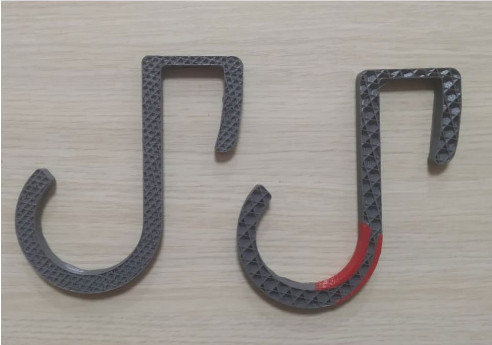
Figure 4. Printed specimens: standard infill (left) vs smart infill (right).
